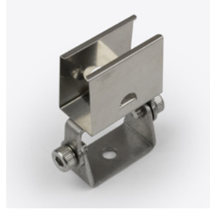
KKBK-24 Adjustable bracket (allow 2 per metre/40in) S/Steel finish L36.5/W13/H41.7mm (L1.44/W0.51/H1.64")
